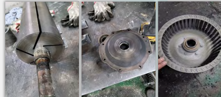
After detecting abnormal signs of bearing, replace the motor.
