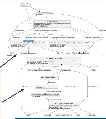
The whole datasheet becomes a graph/model/IDO ontology for the equipment and processes that the datasheet describes
