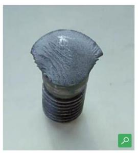
The U.S. Bureau of Safety and Environmental Enforcement has warned the oil and gas industry of a recurring problem with connector and bolt failures in various components used in risers and subsea blowout preventers used in offshore operations.
